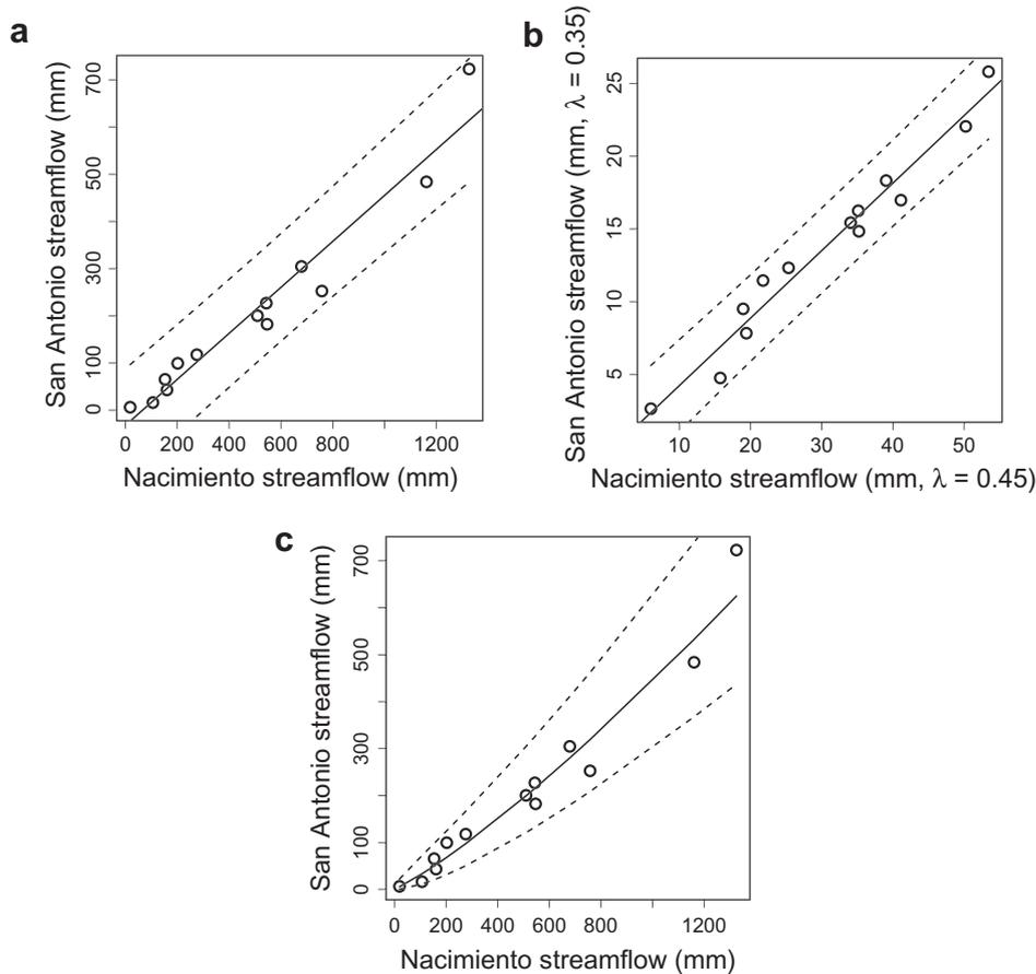
**Fig. 1.** Pre-fire regression model and prediction intervals (dashed lines) for test catchment San Antonio and control catchment Nacimiento for annual streamflow using: (a) original streamflow data, (b) Box–Cox transformed streamflow data and (c) Box–Cox transformed streamflow data translated back into original streamflow units.
