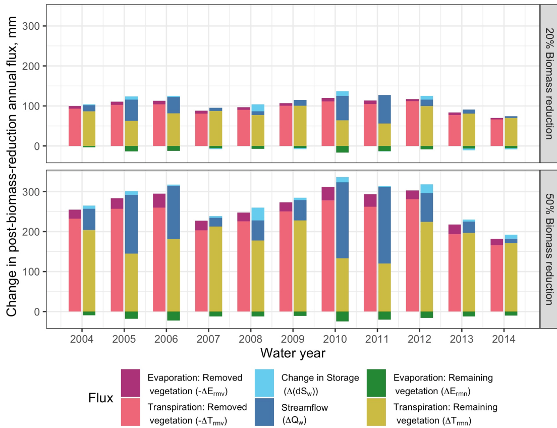
Figure 4: Amount and source of annual water made available from biomass reductions (left bar) and the partitioning of that water (right bar) for each water year averaged over all watersheds for the 20% and 50% biomass-reduction scenarios. The total change in the left bar is equal to the total change in the right bar.
